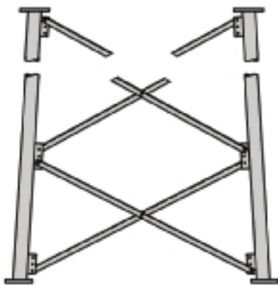
Bracing Detail for Tapered Sections 6SR - 16SR Solid Round Legs & Angle Braces
